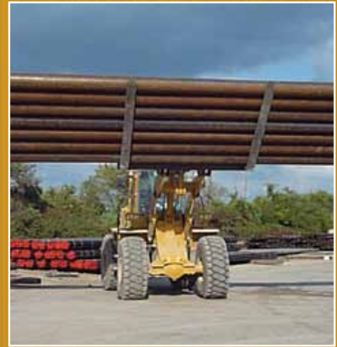
The company's 70ZV-2s use an extra counterweight and 96-inch forks.
