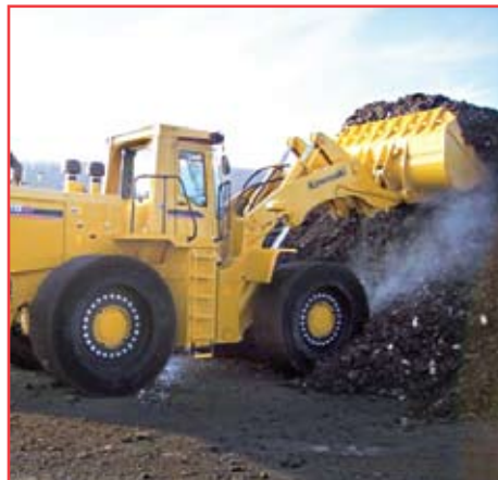
Kawasaki 115ZV-2 wheel loaders keep the company’s Sennebogens supplied with scrap.
