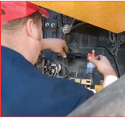
Use Kawasaki's KLEW oil-analysis testing before the loader goes back to work.
