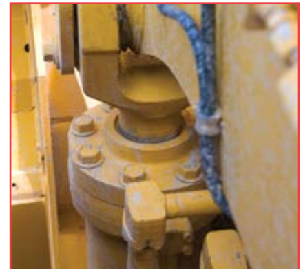
Retract cylinders as much as possible to minimize exposure to the elements.
