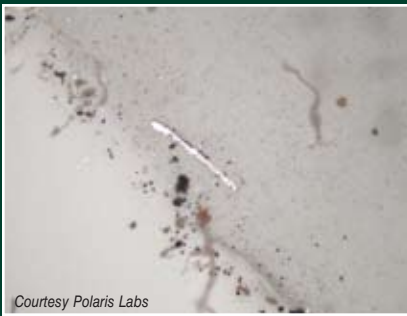
The silver, sliver-like particle measures about 200 microns and is evidence of sliding wear — particles have been magnified 100x.
