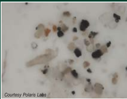
The black particles measure about 15-20 microns — the lighter-colored, fibrous-looking particles are about 30-40 microns (magnified 500x)
