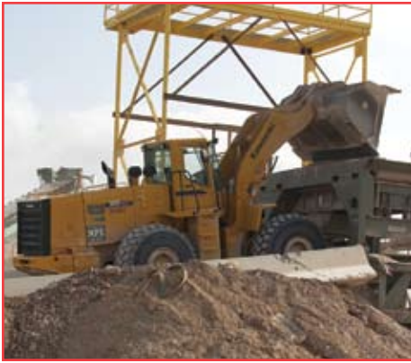
Varmicon uses its 95 for a variety of tasks including feeding the crusher, push-up work (in place of a dozer), maintaining roads (in place of a dozer or grader), and reclamation work.
