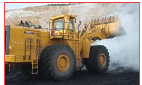
The 135ZV-2 is mainly responsible for the excavation of raw materials for cement, limestone rock, and clay, from a blasted bank.
